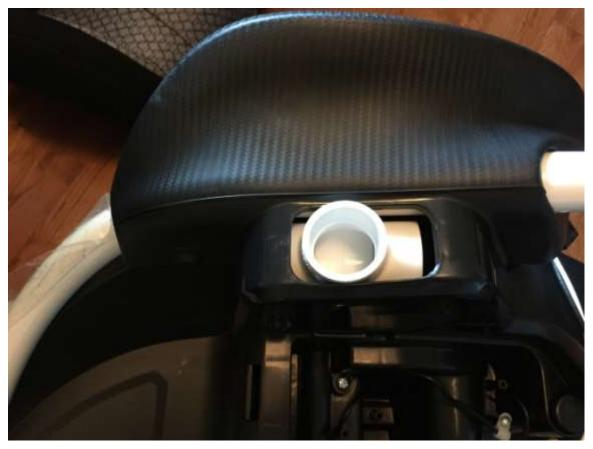
Replace the cover- you will need to pry the top part of the T thru the rectangular hole.
