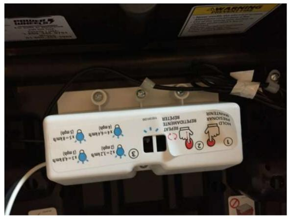
Remove the 4 screws holding the while controller box cover
