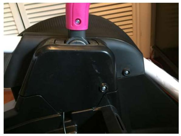
Remove the 2 screws on each side holding the pick controller handle.
