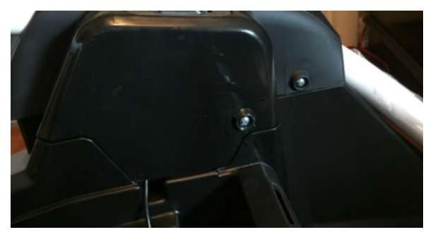
Replace the 2 screws on either side of the cover. Then flip the wild thing over and replace the 4 screws on each side holding the cover in place.
