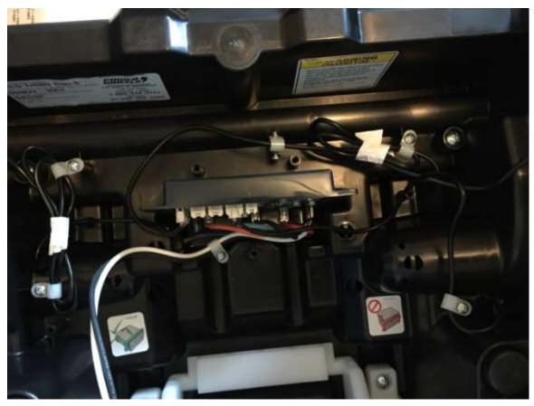
Remove the remaining screws holding the control unit to the base.
