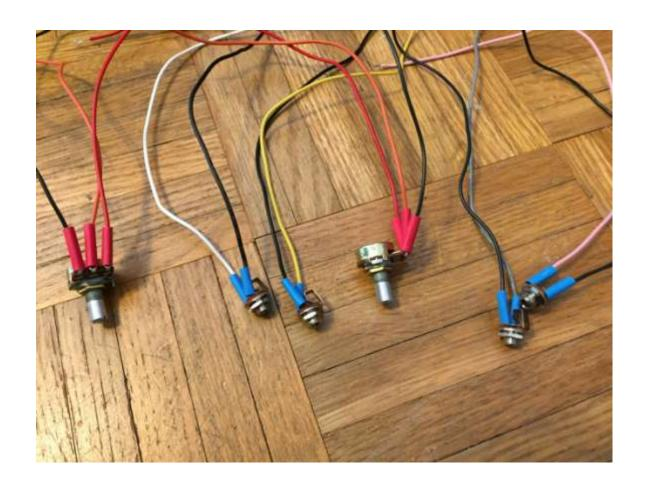
Add heat shrink to wires to cover connections
