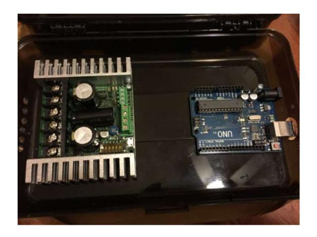
Affix the motor driver and Arduino to the lid of the box. Affix the jacks and potentiometers.
