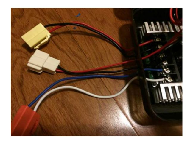
Attach to the sabertooth the 2 sets of wires that will go to the motors. I like to use the 2 blade connectors, and have them color coded to avoid errors. On the Wild thing, you will use spade connectors instead.
