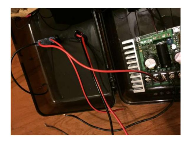
Plug the wire from Batt + of the sabertooth to the middle of the on/off switch.
