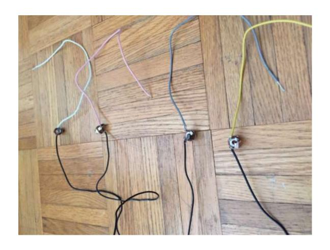
Thread the wire thru the connectors on the mono plug, staying consistent on which will be ground and which connector will be positive
