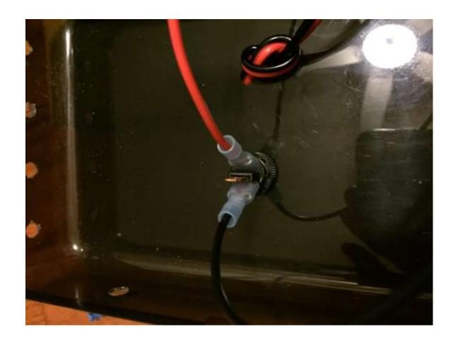
Now it is time to wire Take the black and red wires that you added the quick disconnects and place on the corresponding paddles of the switch
