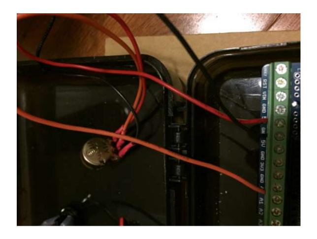
Take the (+) power wire from the potentiometer and attach to the 5V of the Arduino. Take the (-) wires and attach to a ground port. Finally, take the middle signal wire and attach one to AO. Mount the pot thru it's hole and add the nut to affix.
