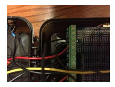
Now take 3 18-20 AWG wires (approx. 12" long). Attach the first from the motor driver (0V) and attach to a ground port on the Arduino. Attach another between the motor driver (5V) and the VCC on the Arduino. Attach the last between the motor driver (S1) and the Arduino digital pin 11.
