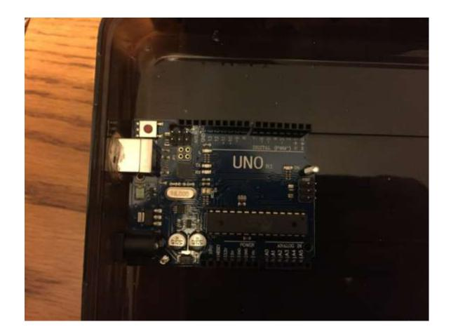
Prepare the box for equipment. Place the motor driver and Arduino in the top of the box and mark where the holes will need to be drilled to mount it. Make sure to mark on the end with the motor driver where holes will need to be drilled for the wires.
