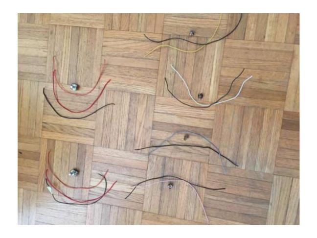
Get and strip the ends off of 22 AWG wires. I like to color code the wires to better identify them. You will need 2 for each of the four mono plugs, and 3 each for the 2 potentiometers.
