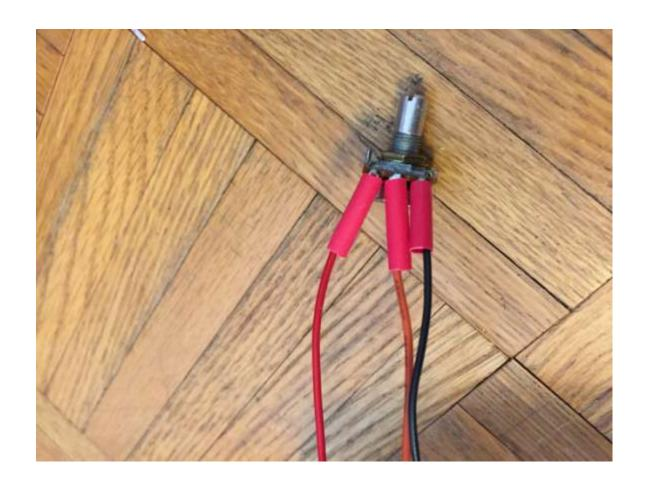
Put shrink wrap on connections and heat with heat gun
