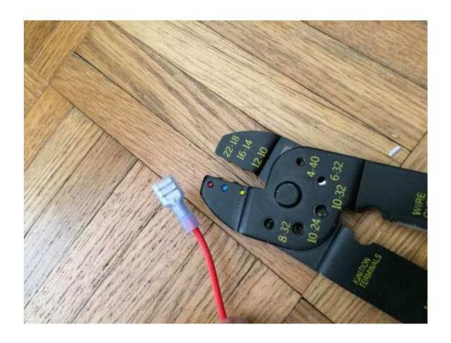
Affix the connectors to the ends of your 3 wires for the on/off switch, leaving one black wire without a connector,
