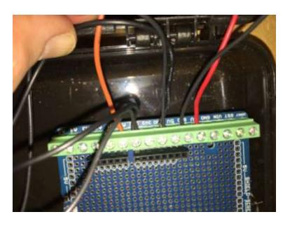
Take 2 of the ground wires from the jacks and attach to a GRN port. Take the other 2 of the ground wires and attach to a different GRN port.
