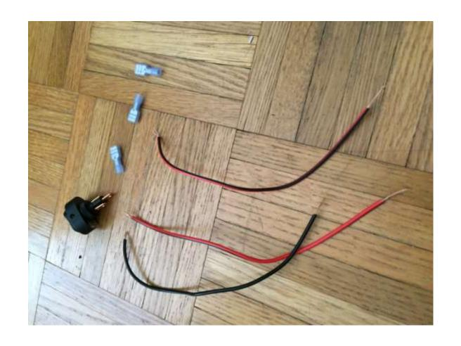
Using 16-18AWG wire, cut 12" portions (2 red , 2 black). Strip the ends. Get 3 insulated connectors.
