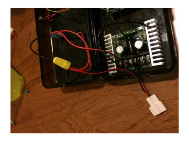
Now take the red wires going into the on/off switch (at bottom), the charging port, and the red wire that will come from the battery and wire nut together. Re-inforce with hot glue
