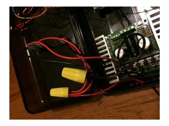
Take the extra black wire that you wired in to the sabertooth, and connect it with a wire nut to the black wires from the on/off switch, the charging cable, and the cable going to the battery
