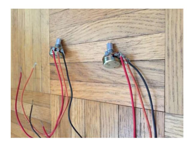
Thread wires thru connection points to prepare to solder
