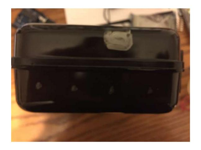
Next mark the holes on one end of the box for the 4 jacks (1/4 drill bit), and then on the bottom section for the 2 potentiometers (9/32 drill bit).
