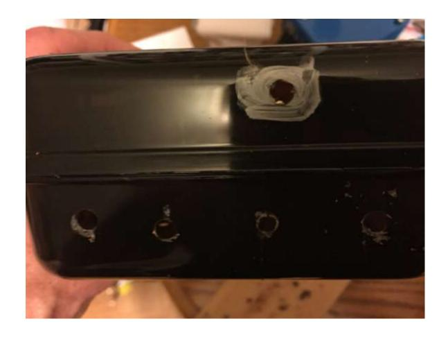
Drill all holes, using a piece of wood to drill into, so you do not splinter the plastic. For larger holes, drill a smaller pilot hole and then use a forstner bit to make the bigger hole.
