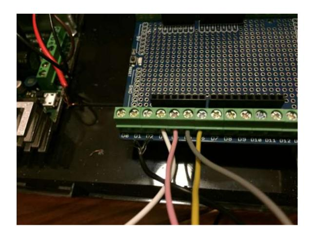
Now attach the signal wires from the jacks to the Arduino, pins 3,4,5,6. (directions......)
