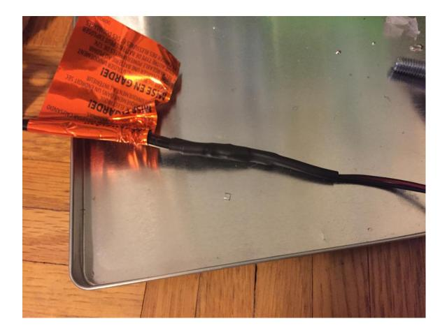
Then pull the last piece of heat shrink over the 2 soldered wires and heat.
