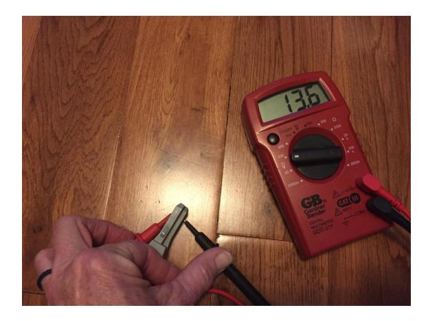
If you are unsure which is positive or negative, use you multimeter to check. Plug the cable into the wall. It should read approx 13.5 when you touch the (+) and (-) plates on the plug. You can also do this after you cut the plug off the cable, but be careful not to let the wires touch.
