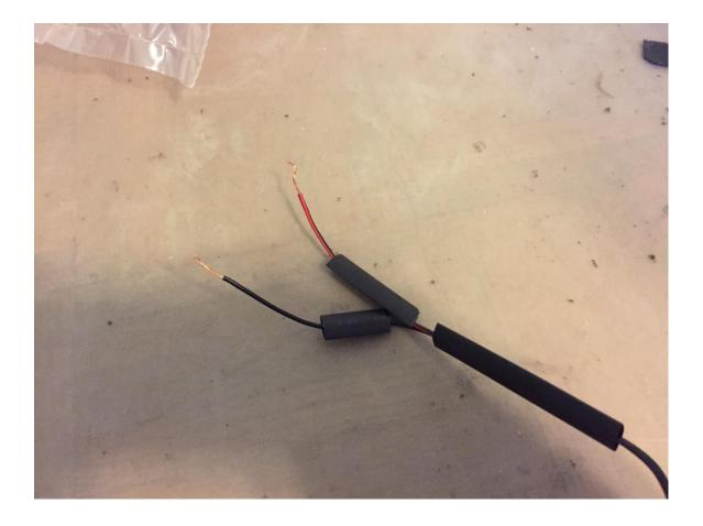
Then thread a piece of heat shrink on each individual wire.
