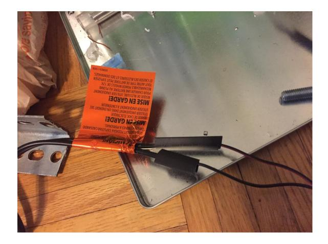
Pull on the soldered wires when cool to make sure you have a good connection. Then cover the 2 wires with the heat shrink.
