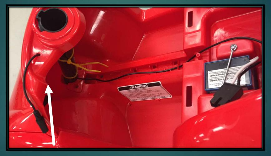
Secure Audio Cord onto Steering Colum and use 2 Wire Ties to Secure
