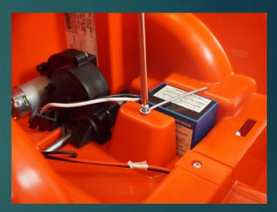
Unscrew the center screw to release the battery
