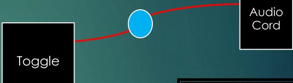
Due to Small Gauge of Audio Cord Wire Immediately Electrical Tape This Connection
