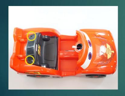
Using a phillips screw driver, remove the 2 screws at the top of the seat
