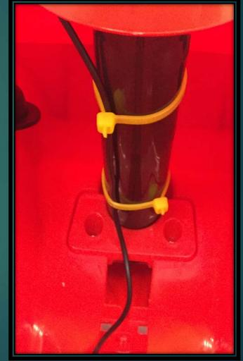
Cut Excess with Plyers or Scissors- do not leave sharp edges.
